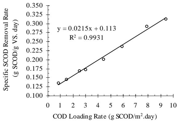
Fig. 3: Relationship between the SCOD loading rate and the specific substrate utilization rate
