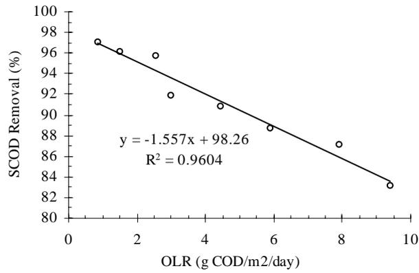
Fig. 2: Effect of OLR on COD removal efficiency
