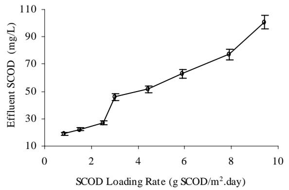
Fig. 4: The effluent SCOD variation with OLR
