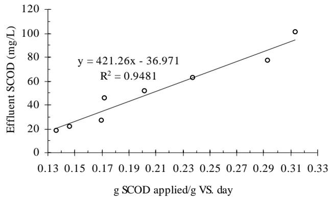
Fig. 5: Effect of specific organic loading rate on the effluent SCOD
