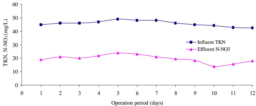
Fig. 12 : Denitrification efficiency in extended aeration activated sludge system
