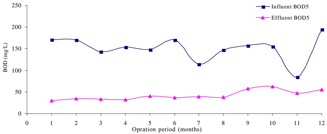
Fig. 5: BOD<sub>5</sub> removal efficiency in extended aeration activated sludge system (Ekbatan WWTP)
