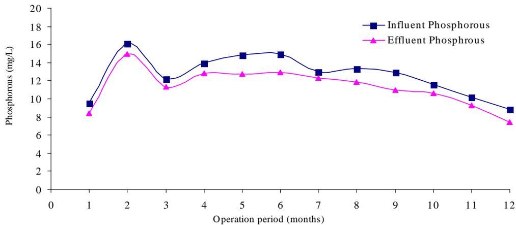
Fig. 8: Phosphorous removal rate in Extended Aeration Activated Sludge System (Ekbatan WWTP)
