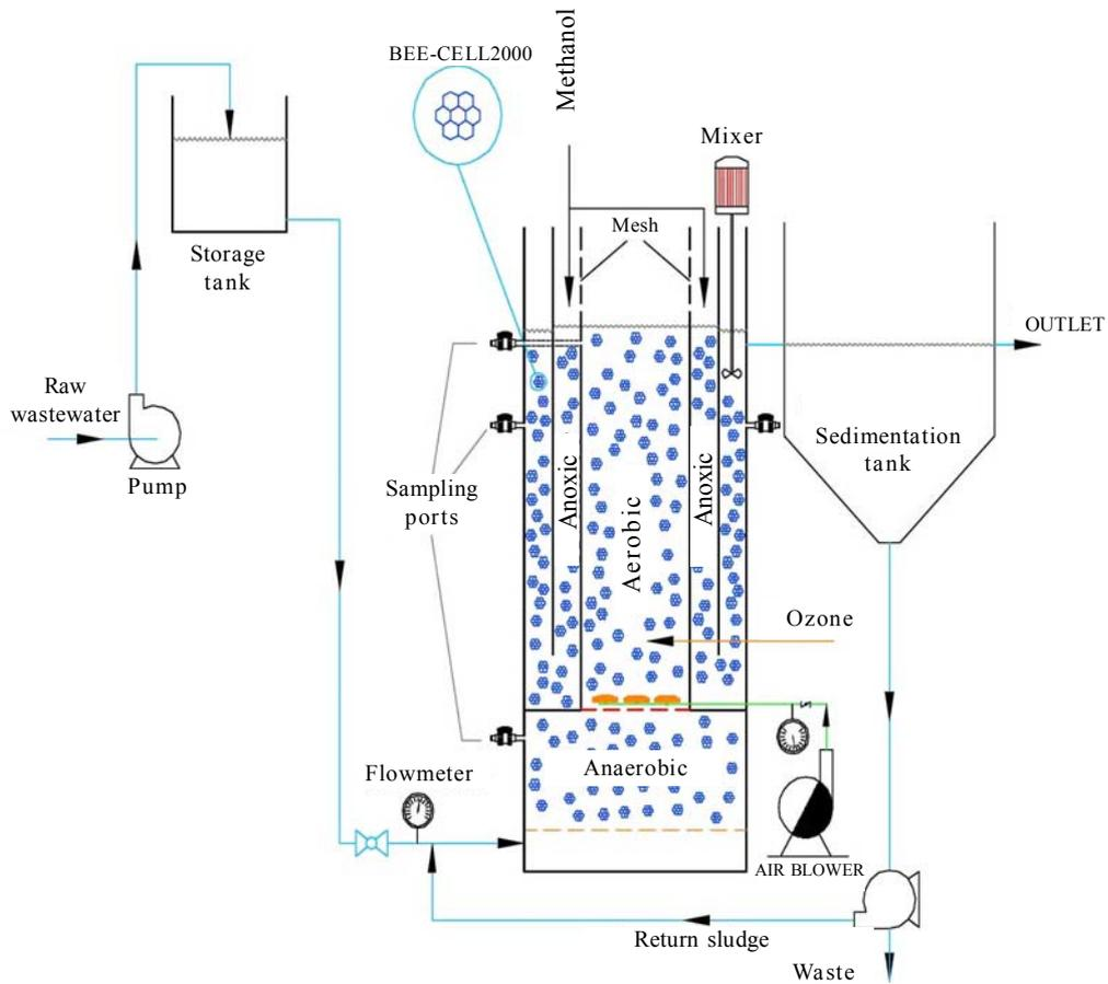
Fig. 1: The schematic diagram of the H-IFAS pilot-plant
