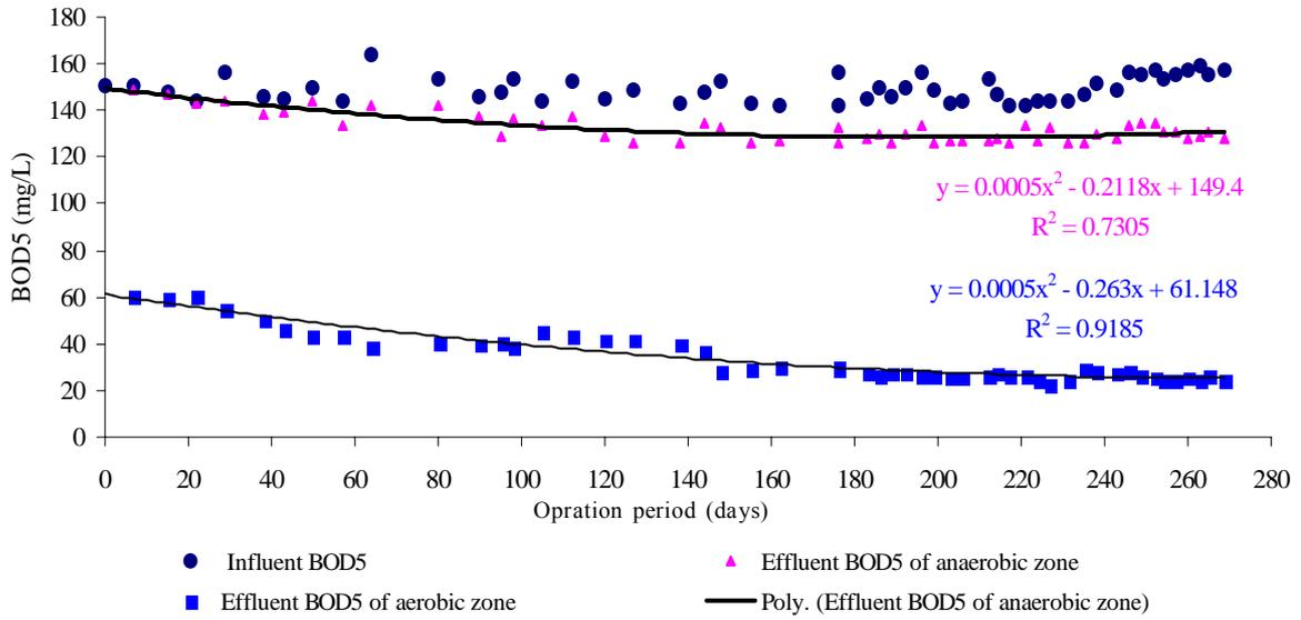
Fig. 4: BOD<sub>5</sub> removal efficiency in aerobic and anaerobic zones of H-IFAS reactor
