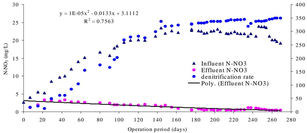
Fig. 11: Denitrification efficiency in anoxic zone of the H-IFAS reactor
