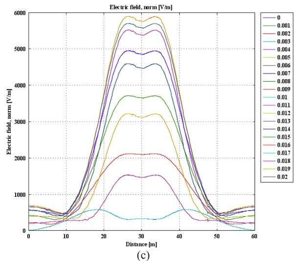
Fig. 4: Electric field intensity for 230kV, 2-circuted DC-type towers according to Fig. 2a right arrangement (a) at  $t=2\text{ms}$  and at 20 time partitions in a period at 2m above the ground according to Fig. 2a right (b) and left (c) arrangements.
