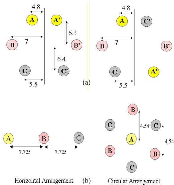
Fig. 2: Phase arrangement of DC type (a) and horizontal and circular types (b), 230kV overhead lines (all values are in meter)
