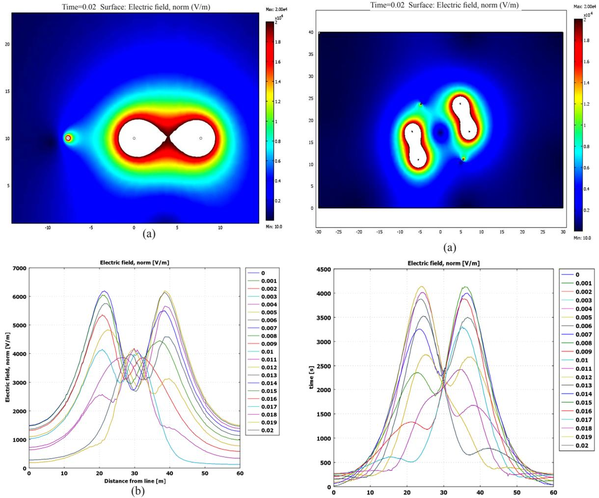
Fig. 3: Electric field for 230kV, SC-type towers at  $t=2\text{ms}$  (a) and for 20 time partitions in a period at 2m above the ground (b). (Intensity of electric field in the white areas of (a) is higher than the maximum determined threshold)
