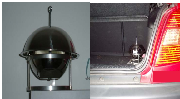
Fig. 2: Illustration of passive samplers in a car boot
