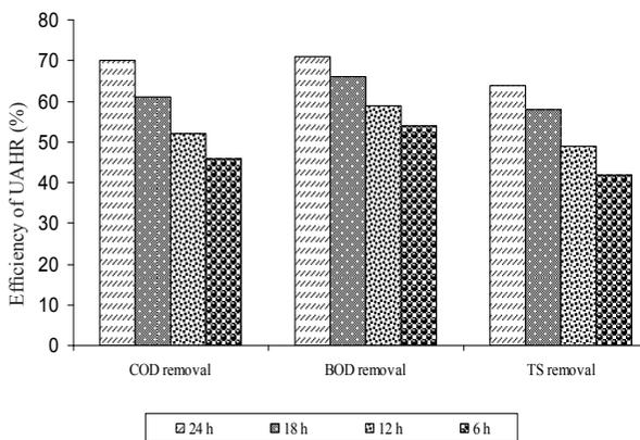
Fig. 2: Effect of Hydraulic Retention Time (HRT) on efficiency of UAHR
