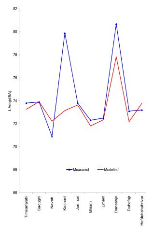
Fig. 6:Comparision between measured and modelled values LAeq
