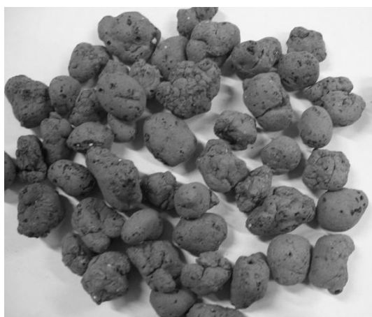
Fig. 2: Carrier Light Expanded Clay Aggregate (LECA) with a density of 0.55 g/cm 3
