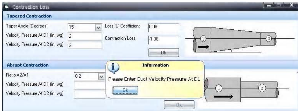
Fig. 8: Contraction and Expansion loss section
