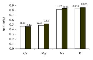
Fig. 4: The effect of other metals on chromium adsorption capacity (Cr= 2mg/L; 2mol/L of Ca<sup>2+</sup>, Mg<sup>2+</sup>, Na<sup>+</sup>, K<sup>+</sup>)
