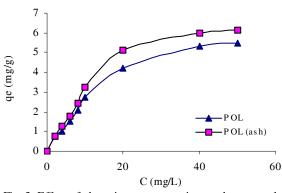
Fig. 3: Effect of chromium concentration on the removal of chromium (VI) by POL and their ash (adsorbent dosage=2g/L; pH =7; T=24°C; 300rpm; 120min)
