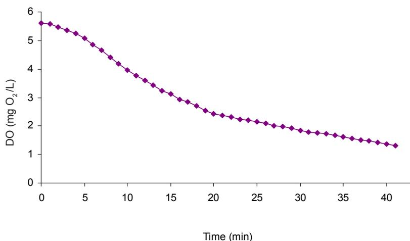
Fig. 6: DO reduction with time under thermophilic conditions
