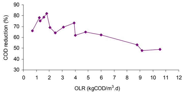
Fig.11: COD removal efficiency versus OLR in MBBR
