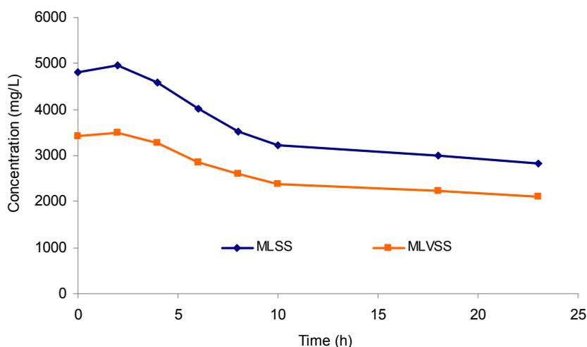
Fig. 3: Changes in biomass concentration during the aeration of activated sludge at 50°C
