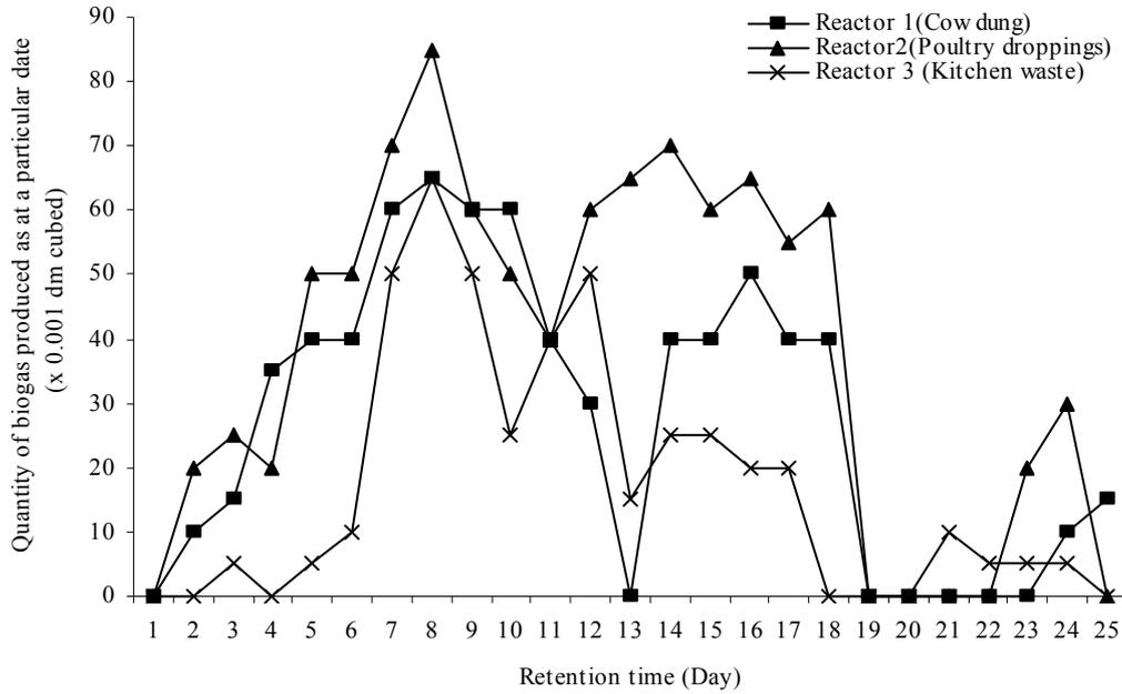
Fig. 1: Biogas production from cow, poultry and kitchen wastes
